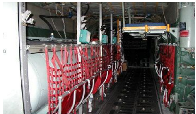
Fuel tank, on left, in cargo bay
