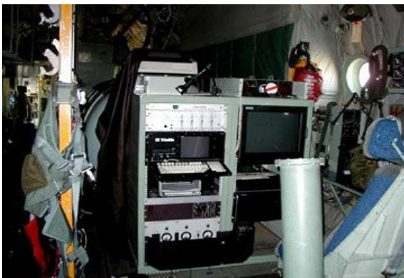
Dropsonde position with launch tube
